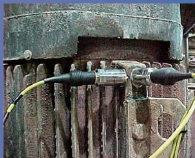
Example of mounting sensors on a vertical type centrifugal pump
