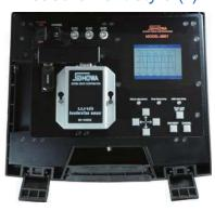
Measurement while monitoring waveforms in real time is enabled.
